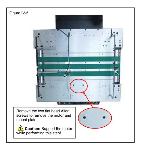
Support the motor and motor mount plate while removing the flat head Allen screws as indicated in step A.
