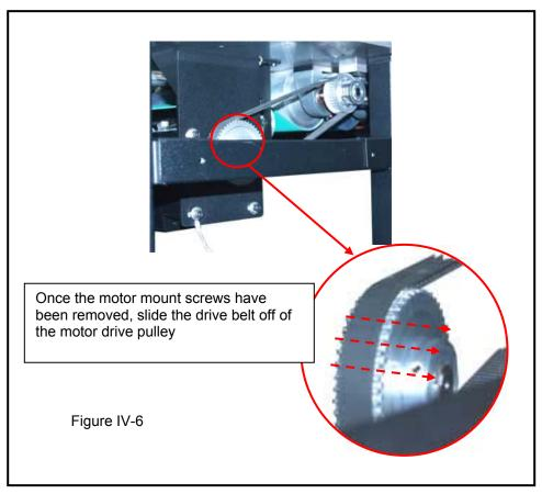
With the Power turned off and the power supply disconnected from the machine, it is not necessary to disconnect the power supply to the motor after lowering the motor to the bottom of the machine base. If you choose to disconnect the power cable to the motor, perform the following:
