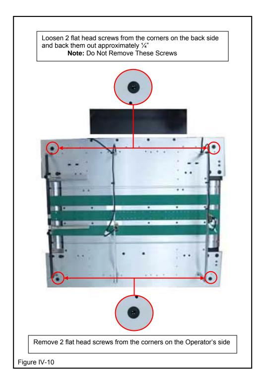
H. Lift the front edge of the transport belt top plate assembly up approximately 1" from the vacuum base and slide the old belts, one at a time, towards the front (Operator's side) to remove them, see figure IV-11.
