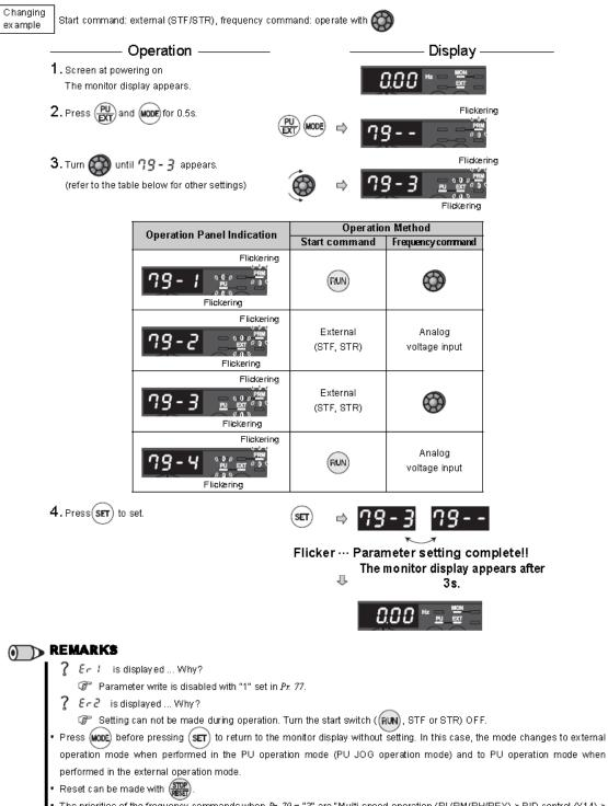
The priorities of the frequency commands when P: 79 = "3" are "Multi-speed operation (RURM/RH/REX) > PID control (X14) > terminal 4 analog input (AU) > digital input from the operation panel".
