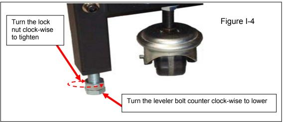
6. Place a level in the center of the FIT 36base and adjust the leveler pads as needed to level the machine at the desired height. Once the machine has been leveled, tighten the leveler pad lock nuts, see figure I-5.
