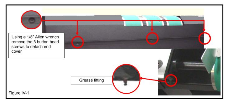
Α. Detach conveyor end belt guard(s) by removing (3) button head screws, see figure IV-1.
