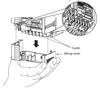
Also pull the wiring cover downward with holding a frontal part of the wiring cover.
