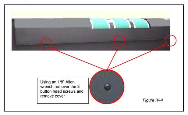
Remove the motor and motor mount plate by performing the following;
